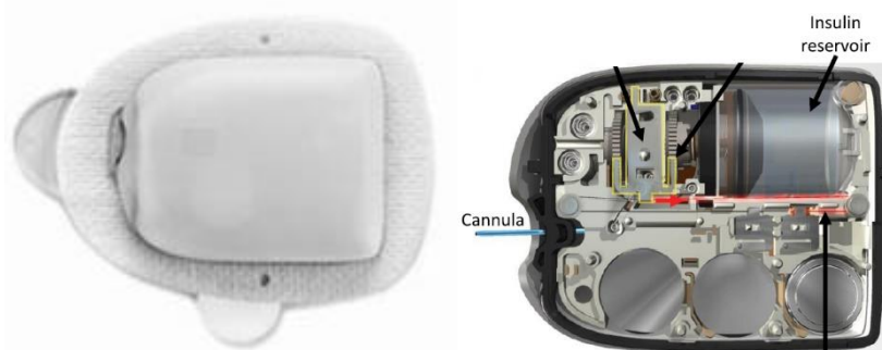
Figure 2 Omnipod Dash patch insulin pump (external and internal)
